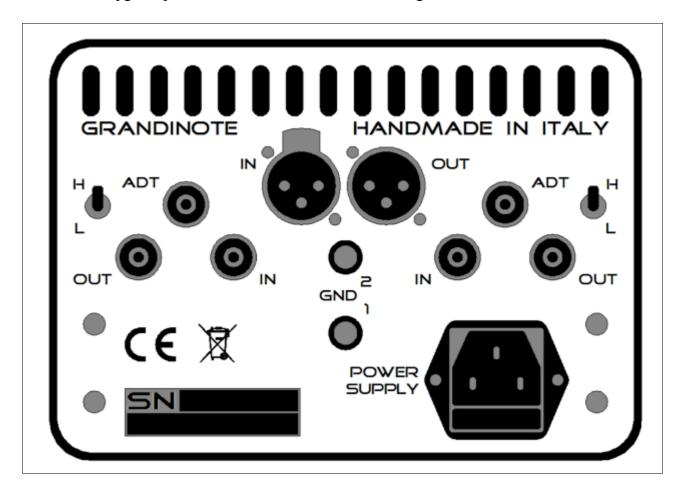
Both input RCA stereo signal or XLR mono signal are subordinate to loading adjustment. Upon order one can specify needed cartridge loading and Grandinote will prepare the calibrated external RCA ADT connectors to match the spot on impedance loading.
