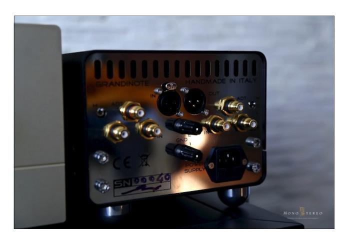
Additional gain switch with L and G lock gives more option and translates to low and high gain adjustments, helping to match the optimal gain loading to the line preamplifier. Nearby additional two ground connectors GND 1 and GND 2 are serving for device "body" and signal ground, opening up the doors for experimentation with the proper noise level.
